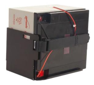
The BP24 requires a regulated charging source (provided by the CH100 or CH200 regulator connected to an unregulated solar panel or a wall charger). The BP24 includes a 12 in. cable that terminates in a connector for attaching the battery to a CH100 or CH200 regulator. The BP24 is shipped with a bracket that secures the BP24 to an enclosure back plate. An ENC16/18 enclosure is recommended.
